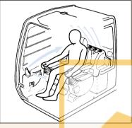
Air conditioning and a "Hot and Cool" box are standard on the EX200. The large capacity unit features front and rear rotatable louvers. Automotive-type controls blend hot and cold air to provide the perfect temperature.
