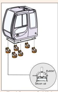
The cab floats on six fluid-filled elastic mounts that smooth out shocks and jolts.
