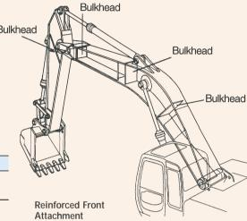
Bulkheads are provided inside the front attachment to resist torsion and thickened plates are used in areas subject to stress concentration for added durability in tough operations.
